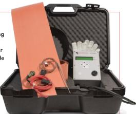
ite decking. Heatcon responded by developing a heat-forming kit for decking based on the same heating-blanket concept as the trim-bending kit. Subsequent tests revealed the need for an internal temperature probe to monitor and regulate a slower heating process for the thicker PVC and composite deck boards.
