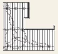
I start by overlaying my design on a deck plan with standard 12-in.-on-center joist framing.
